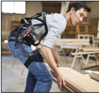
Figure 1: An experimental backX for workers. The torque generators at the hip compensate for the torque due to the upper body weight and therefore minimize the erector spinae muscle forces at L5/S1 location
